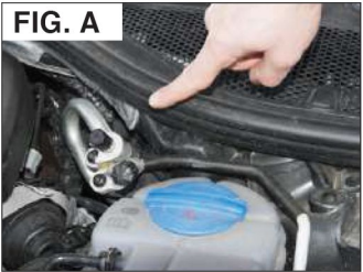
FIG. A 30 mL (1.0 fl oz) UNIVERSAL DOSE for VEHICLE A/C SYSTEM
